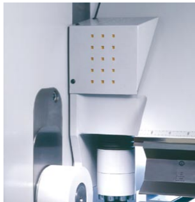
PowerBoosters create 120 metric tons (130 US tons) of pressure. Result: Perfect hems and tight bend radii.
