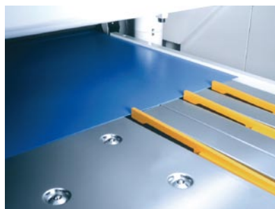
The front or rear pop-up fingers position the part to the programmed dimension.
