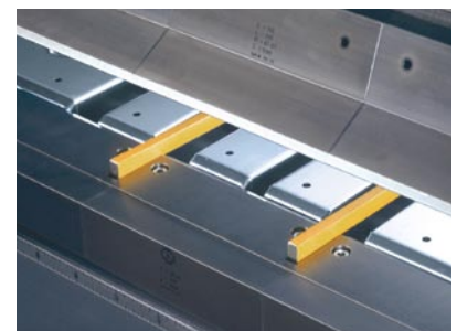
The front fingers can move into the lower beam tool finger pockets.
