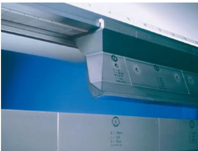
The upper beam tool clamping system automatically locks the tools into place.
