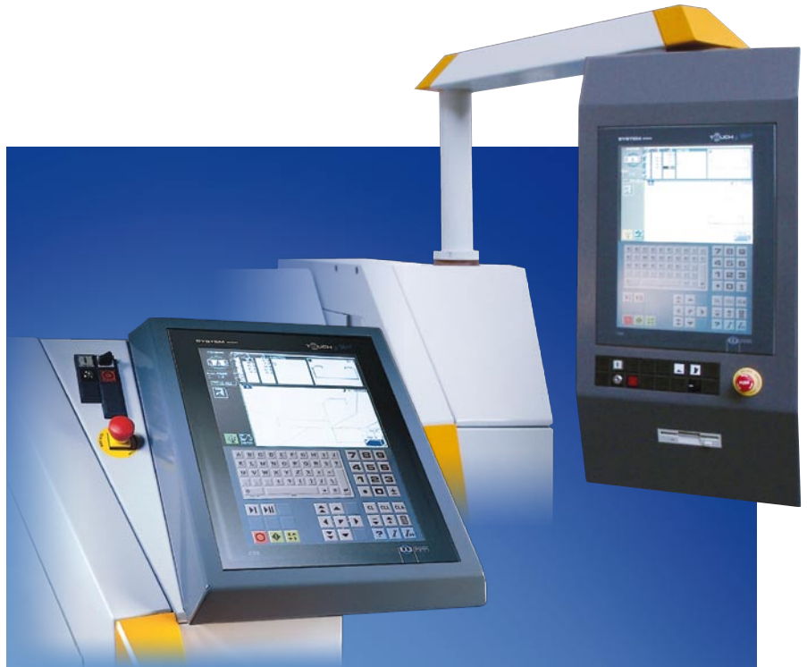
Ergonomically positioned Touch&More control for optimum visibility (Optional: Control on swivel arm)
