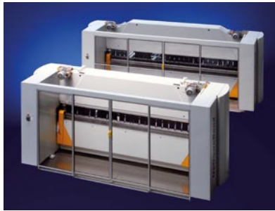
Glass sliding doors secure the folding area
