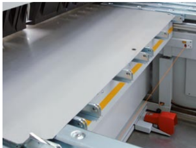
Special gauging system: Visible safety light system
