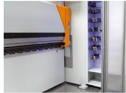
Tool magazine in machine stand
