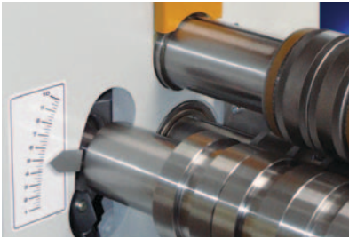
The position indicator allows for repeatable radius adjustments
