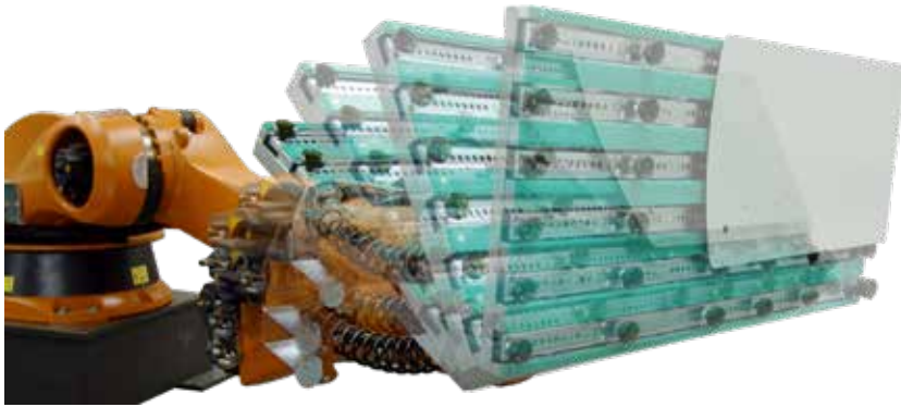
The loading robot flips the blanks.
