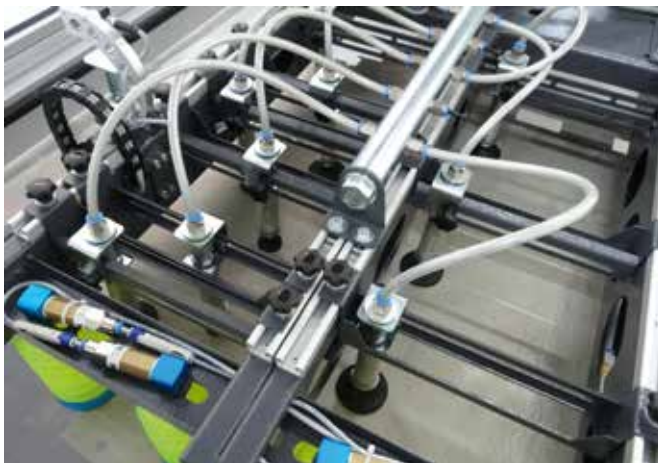
Suction frame of the gantry loader with 6 suction cups used to peel up the blank and 45 freely moveable suction cups.
