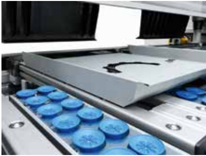
Automatic part positioning by a suction gauging system.
