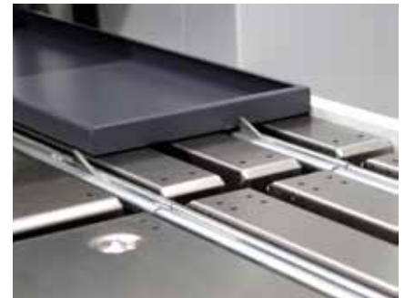
Part lined up with the squaring arm.
