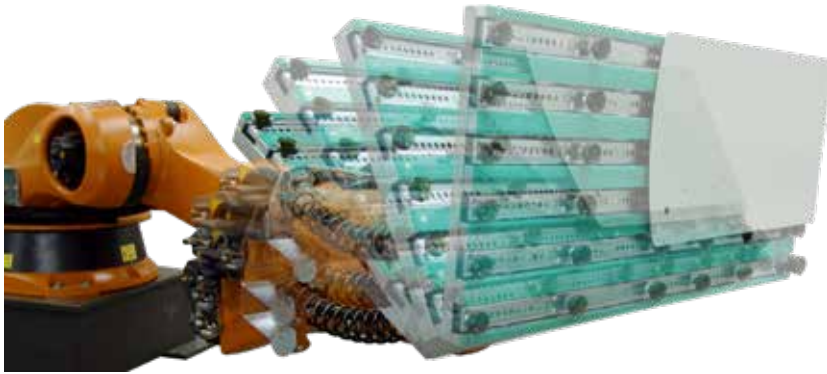
The loading robot flips the blanks.
