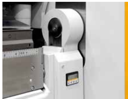
Optional digital display for folding beam adjustment.
