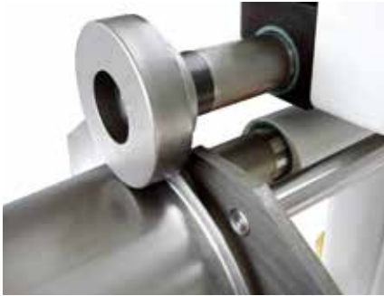
Flanging wheels FL: Flanging without swiveling the part.
