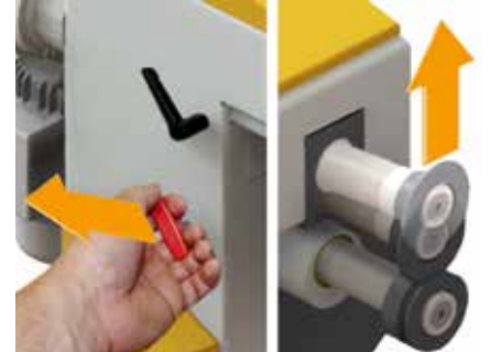
UnLock function opens the wheels immediately in an emergency.
