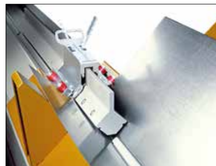
Autopilot and reinforced seaming bar on the RAS 20.12 DuctZipper.
