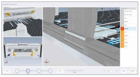
The 3D simulation shows the folding sequence and possible collisions. New products can already be evaluated during the design process.
