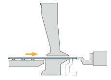
Maximum bending accuracy due to the patented beam-in-beam folding beam design.
