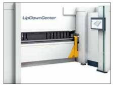
Machine without tool changer. A light curtain combines safety and access while operating from the front.
