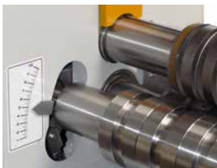
Scale for radius adjustments
