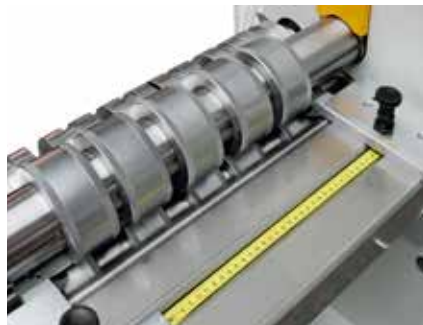
Tape measure for quick roll positioning
