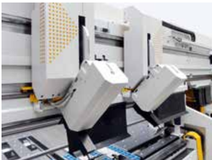
The automatic tool changer places the tools of the upper beam in position.
