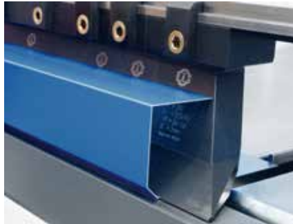
Segmented upper beam tools with front free space
