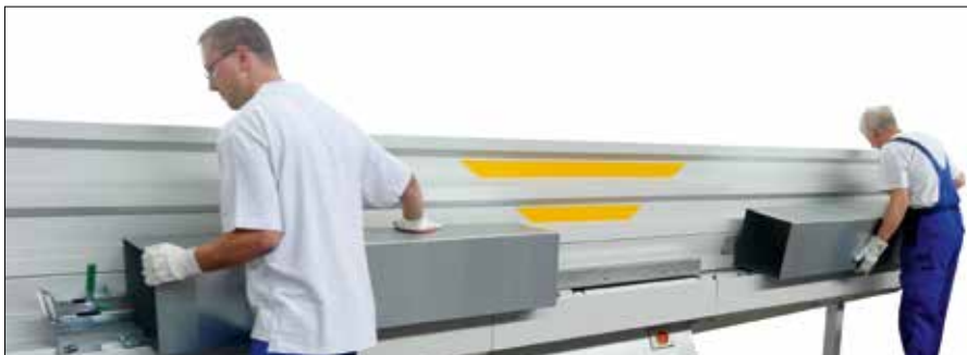
Operating speed doubled: After the first duct is finished and removed, the operator clamps the next duct with the AutoPilot and is ready to pass the next air duct through the machine.
