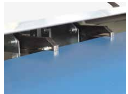
Grippers position the part. This ensures precise flange dimensions and fast bending sequences.
