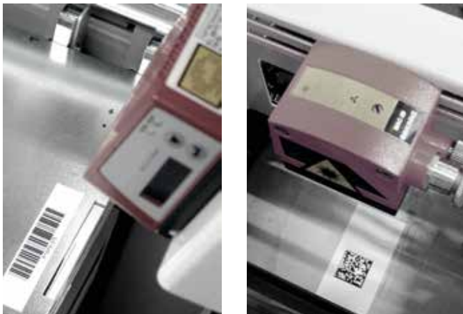
Automatic program loading can be added to the MiniFeeder or gantry loader by scanning a barcode or QR code label on the blank.
