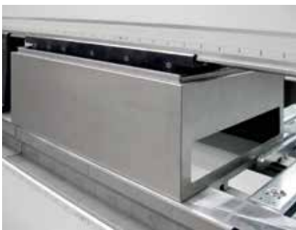
Tall upper beam tools allow the production of deep boxes.
