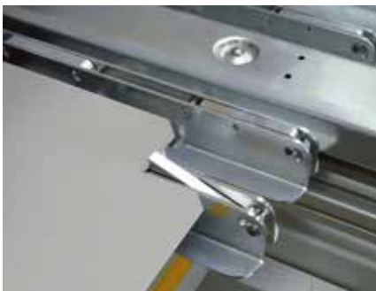
Flexible part positioning. Individual stop fingers can be deactivated.
