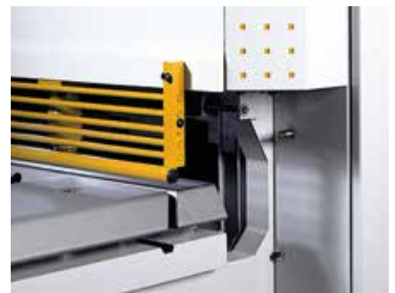
Side free space for an easy blade change
