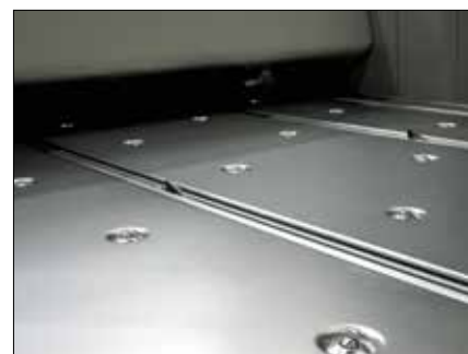
Sheet support tables with ball casters
