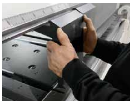
Quick tool set-ups due to the automatic tool clamping system.
