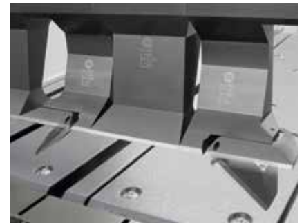
The SnapTool corner tools automatically retract from parts with side flanges.
