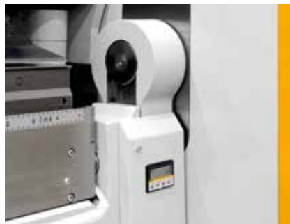
Optional digital display for folding beam adjustment.
