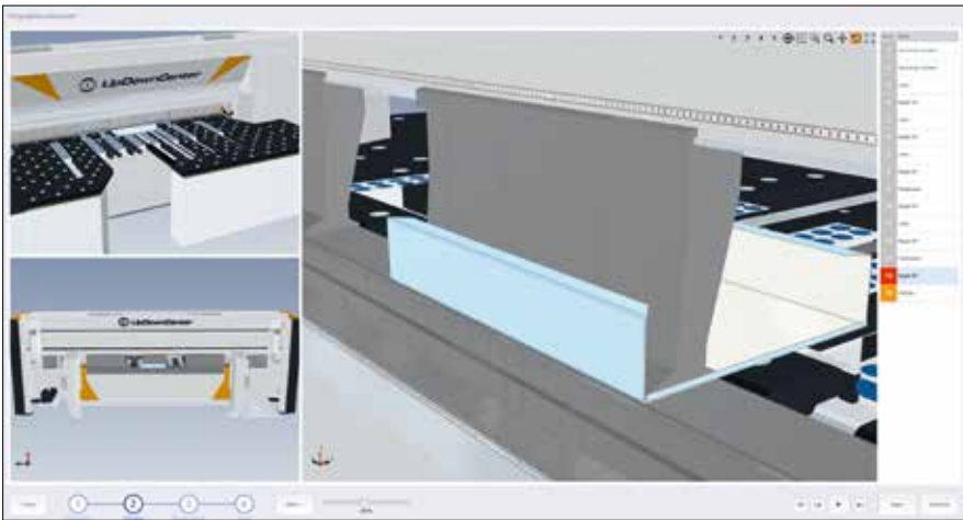
The 3D simulation shows the folding sequence and possible collisions. New products can be evaluated during the design process.
