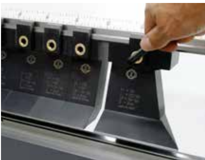
Tools with quick clamping system
