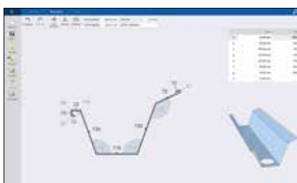
Input of part geometry by drawing, table values input or STEP / DXF file import.
