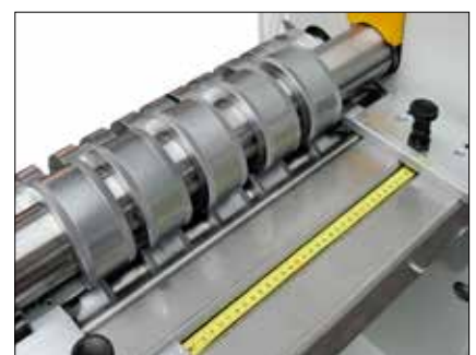
Tape measure for quick roll positioning
