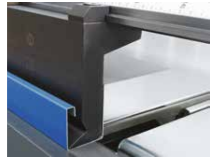
Segmented upper beam tools with rear free space
