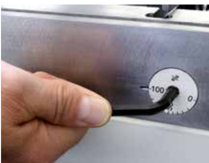
Setting the CrownTool.. (especially for step bending of radii).
