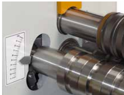
Scale for radius adjustments
