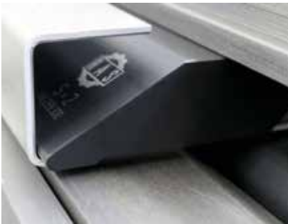
Tools with radius for bending aluminum.
