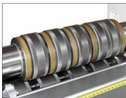
Rolls for standing seam and snap-lock seam.
