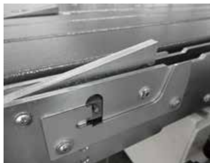
If the outside edges of the blank are not straight, individual stop fingers can be deactivated.
