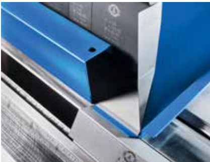
Bend tabs with segmented folding beam tools.
