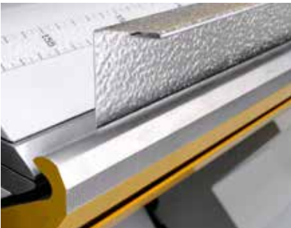
No part rotation required since the machine bends up and down. High productivity due to fast bending cycles.
