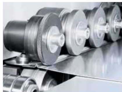
Set of rolls for Pittsburgh seam
