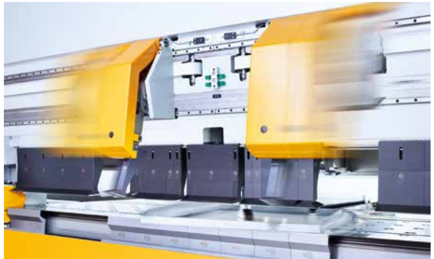
Fully automatic bending sequences: positioning, rotation, bending, and tool change.
