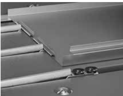
The suction cups of the hybrid gauging system hold the part through a sequence of bends to the stop fingers.
