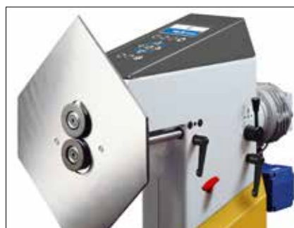
Stop plate for insulation pipes
