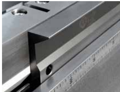
Part design flexibility due to slim but rigid folding beam tools.
