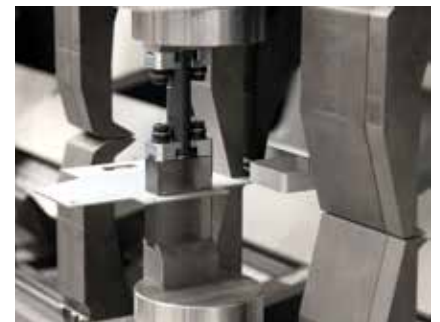
Several bending stations can be setup along the length of the machine. Complex parts can be completed in a single run.
