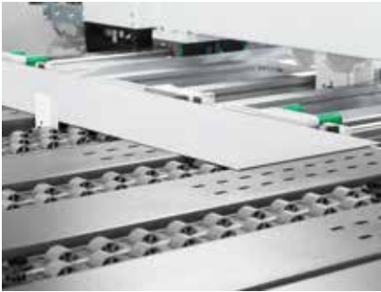
Secured bending accuracy due to automatic alignment of the supplied blanks.
