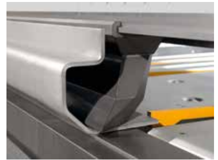
Upper beam tool with large front free space.
