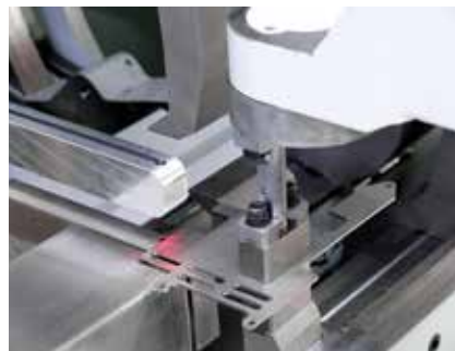
Measuring the parts by a laser scanner.
