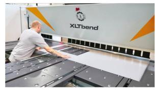
Due to the variety of different sheet dimensions, production batch sizes are small. Head of design Michael Roy explains: "We have stored the most important geometries of our panels in the machine software and usually only change the length and width of these components.
