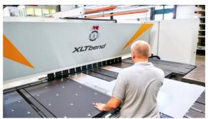
Working from the center of the machine also contributes to the precision of the bent parts. A central stop finger extension increases the standard stop dimensions from 1550 mm to more than 4000 mm. The center working orientation creates an even force curve in the bend, leads to extremely straight bends and reduces the stress on the machine. An additional squaring arm close to the center of the machine simplifies gauging of long and narrow parts.
