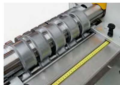
Tape measure for quick roll positioning.
