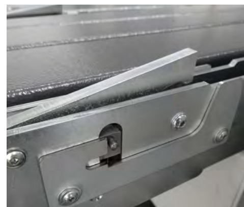
If the outside edges of the blank are not straight, individual stop fingers can be deactivated.
