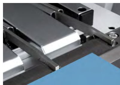
Stop finger at minimum stop dimension.
