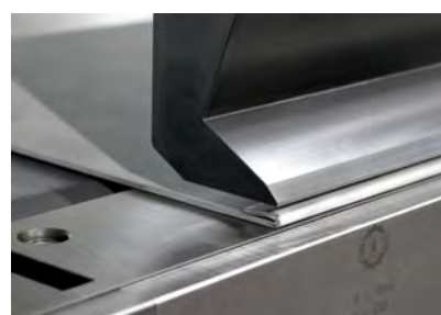
The PowerBoosters offer impressive performance when hems need to be closed.
