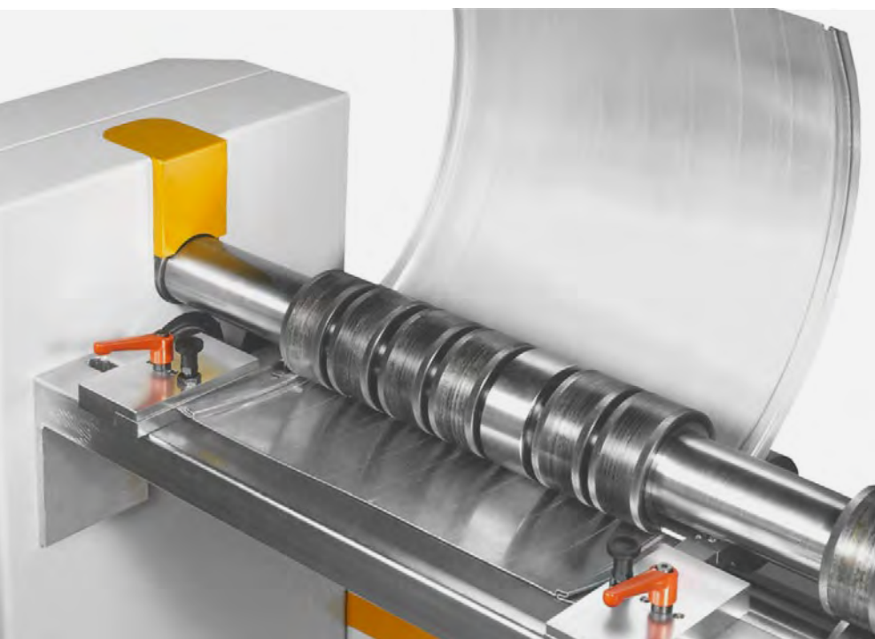
Rolls easily adjustable to the width of the part.
