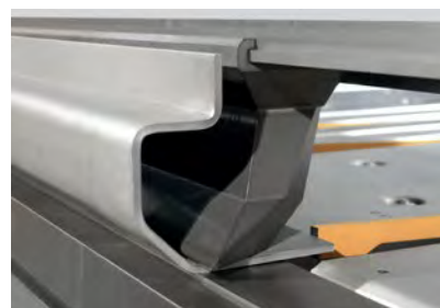
Upper beam tool with large front free space.
