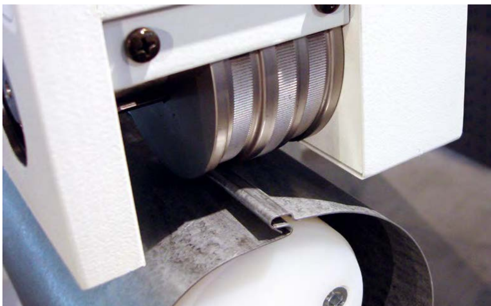
Closing of longitudinal seam (tube seam) on round tubes
